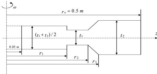
Fig. 8. Rotating disk of flywheel.
