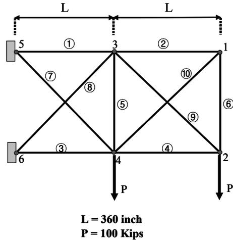
Fig. 7. Ten-bar planar truss.
